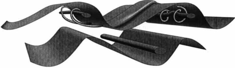
FIGURE 13. Conceptual picture of ribs and spanwise eddies in the near wake.
